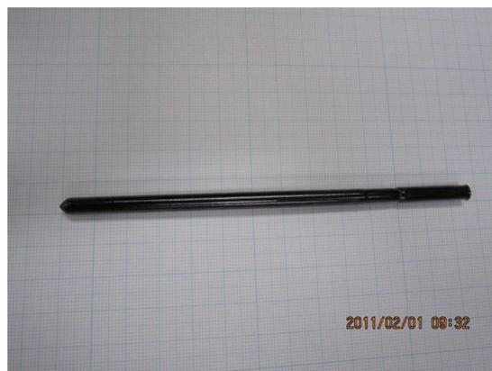
Fig. 2  $\text{La}_{1.67}\text{Sr}_{0.33}\text{NiO}_4$  single crystal
