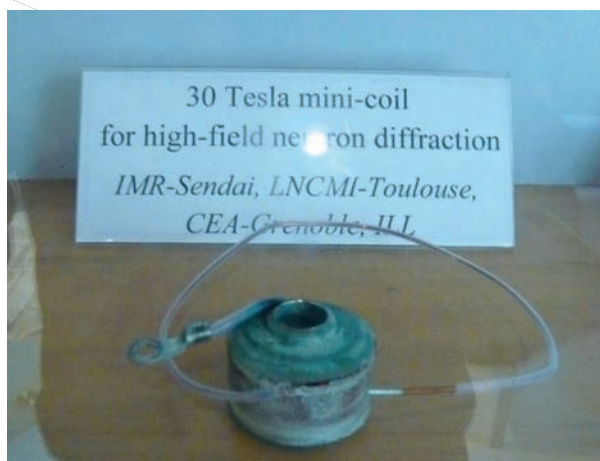
30 T Mini-coil for a neutron experiment
