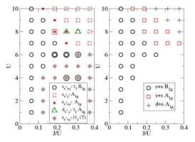
Fig. 1: Pairing phase diagram of the two-orbital model for Fe ions obtained by exact diagonalization on the 8-(small symbols) and 10-site (large symbols) clusters.
