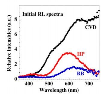
Fig. 4: IMR initial results for radioluminescence characterization of CVD SiC using proton irradiation. Visible and IR regions.
