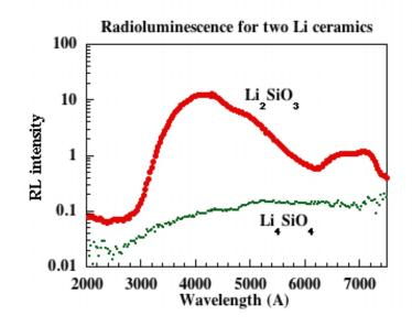
Fig. 2: IMR results for radioluminescence characterization of Li containing ceramics using proton irradiation.
