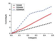
FIG. 2. Current of seven-chain zigzag graphene nanoribbons with/without hydrogenation chains.
