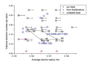
Fig. 1 Compositions of low-*E* alloys in a 2D map coordinated by valence electron concentration and atomic size. The data are both from our experiment ( $\Box$ ) and from the literature ( $\bigcirc$ ). The non-BCC alloys are marked with  $\triangle$ . The Young's moduli *E* below 65GPa are shown near the alloy compositions.
