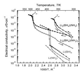
Figure 1: Electrical conductivities of LiBH<sub>4</sub>, LiNH<sub>2</sub>,  $Li_2(BH_4)(NH_2)$  and  $Li_4(BH_4)(NH_2)_3$  (triangle).
