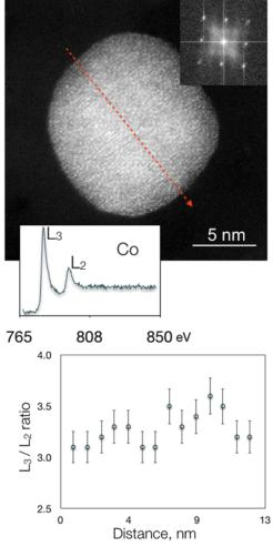
Aberration-corrected HAADF STEM image of a Co<sub>26</sub>Pt<sub>74</sub> alloy nanocrystal. Inset is a fast Fourier transform pattern showing no structural ordering. Background subtracted Co L-edge is shown in the next image that was used to determine the L3/L2 peak ratio along the nanocrystal as marked by red arrow.
