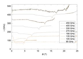
Fig. 2 Antiferromagnetic resonance in Cu<sub>2</sub>OCl<sub>2</sub>.
