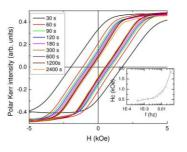
Fig. 1 Dynamic magnetization hysteresis loops of a FePt (5nm) thin film measured by PMOKE.
