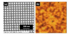
Fig. 2 (a) SEM and (b) MFM images of 25 nm FePt dots with the pitch of 75 nm. The MFM image was observed at H = -3 kOe.
