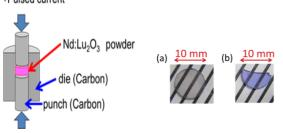
Fig. 1 Schematic view of SPS technique to fabricate Lu2O3 ceramics doped with 0.1 mol% (a) and 5.0 mol% (b) of Nd (after polishing).
