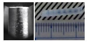
Fig. 1 *In-situ* view of stable growth conditions during the micro-pulling-down experiment and the resulting crystal of KCal<sub>3</sub>:Eu.\_
