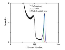
Fig. 2 Gamma-ray spectrum of KCal\_3:Eu showing energy resolution of 3.8% at 662 keV and ~70,000 ph/MeV light output.\_
