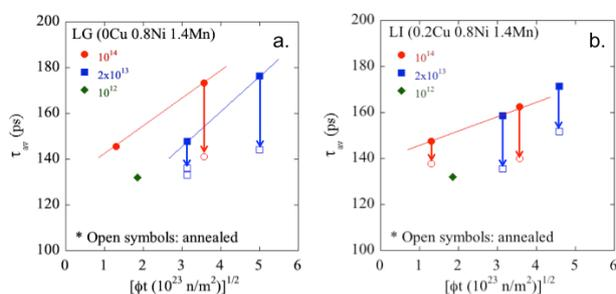
Figure 1 Average positron lifetime ( $\tau_{av}$ ) before (filled) and after (unfilled) recovery anneal versus neutron fluence ( $\phi t$ ) for  $\phi$  from  $10^{12}$  to  $10^{14}$  n/cm<sup>2</sup> in a) low and b) high Cu RPV steels.
