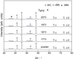
Fig. 2 XRD patterns of WC-40vol%cBN/SiO\_ raw powder and composites consolidated at 1773 to 2073 K  $\,$
