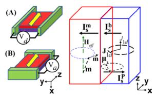
Fig. 3: Schematic spin battery operated by FMR for the measurement configurations (A) and (B). The AC(DC) voltage drops  $V_a$  ( $V_d$ ) along the z(y) direction. In the right panel the magnetization **m** (time derivative precesses around the effective field H<sub>eff</sub> in the left layer, generating DC/ AC spin currents and a spin accumulation in the normal metal (right side) [3].
