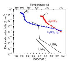
Fig. 2 Electrical conductivities of  $Li_2BNH_6$  and  $Li_4BN_3H_{10}$ . The melting temperatures are indicated as  $T_m$ . For reference, the data of the host hydrides  $LiBH_4$  and  $LiNH_2$  are also shown.
