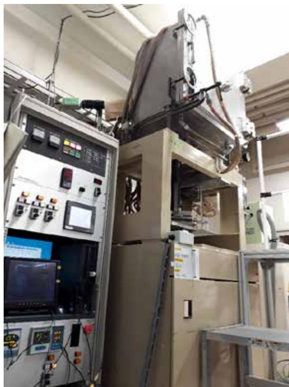
Fig. 1. Photograph of the  $\mu$ -PD growth machine.
