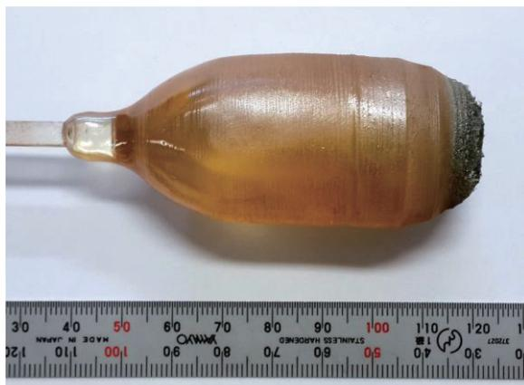
Fig. 2 As-grown  $\text{CdWO}_4$  single crystal
