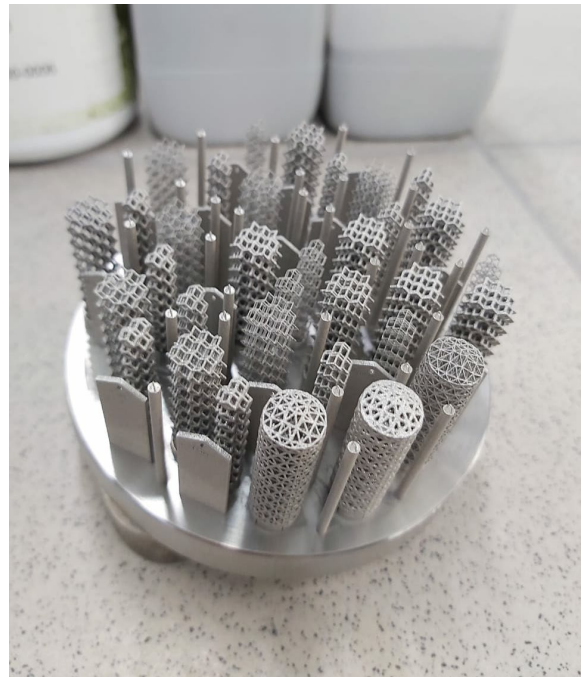
Fig. 1 shows additively manufactured Inconel 718 samples
