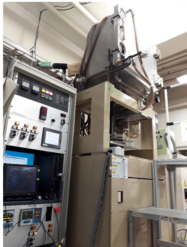
Fig.1. Photograph of the μ-PD growth machine.
