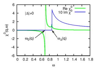
Fig. 2: The blue line is the onset of PH pair creation. As can be seen, gap opening pushes the edge of PHC to higher energies, but leaves behind a simple pole for the real part at the initial edge of the PHC.
