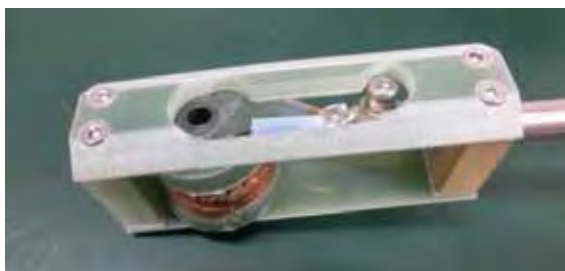
Fig.2 A new 35 T minicoil magnet developed at the IMR facility for THz-TDS measurements at Rice University.
