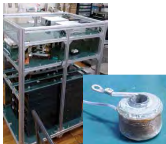
Fig. 1 The mobile pulsed field generator and the magnet used for neutron diffraction.
