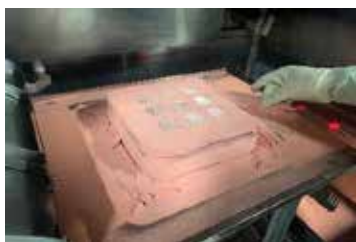
Fig.2 shows the additive manufactured sample in electron beam powder bed fusion machine.
