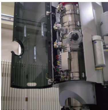
Fig. 1 Cs corrector at the objective lens, which makes the resolution of phase contrast image better than 0.1 nm.
