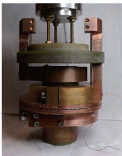
Fig. 3 Photos of (Top) double-stacked RE123 tape co-wound coil at Tohoku University and (Bottom) single tape wound RE123 coil at LNCMI.
