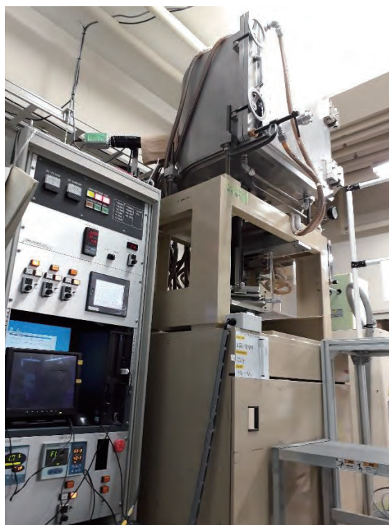
Fig.1. Photograph of the \mu -PD growth machine.
