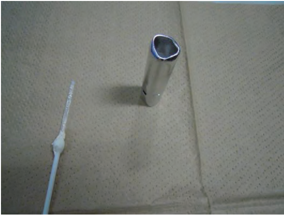
Fig.2. An Ir crucible attached to the after-heater and GAGG seed mounted to the alumina rod.
