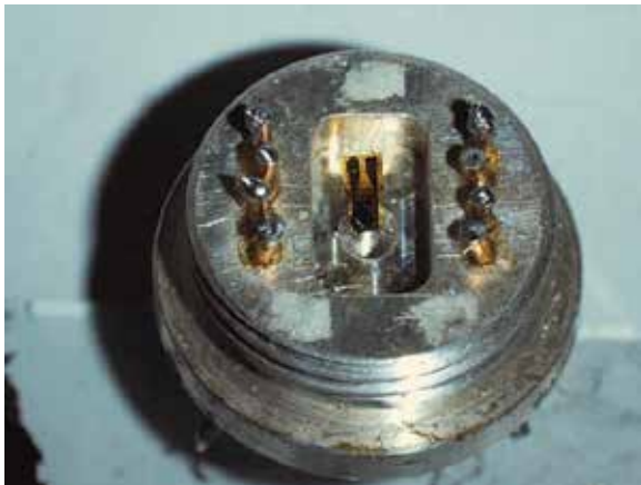
Fig. 2 An example of the sample stage for heat capacity measurement in very low temperature.
