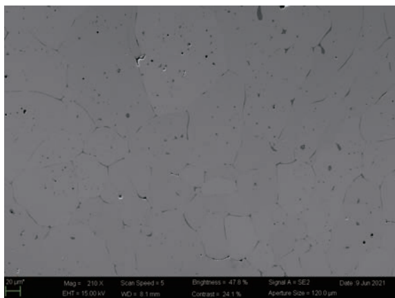
Fig. 1 SEM of Nb-Fe-Al precursors prepared by arc melting
