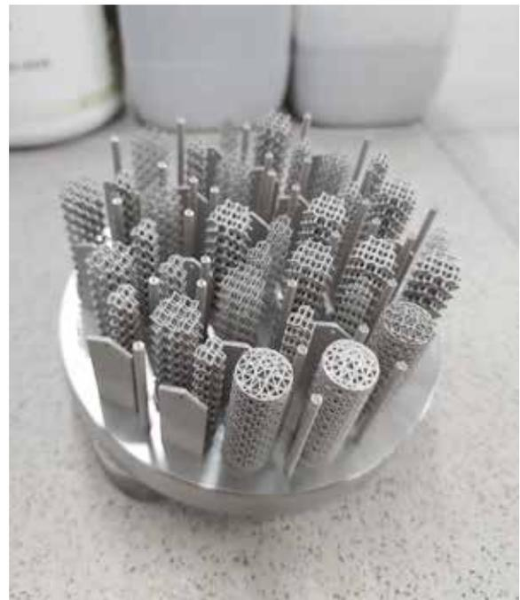
Fig. 1 shows additively manufactured Inconel 718 samples
