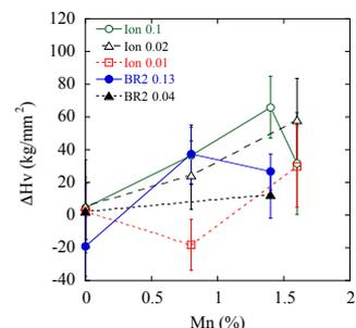
Figure 3 Mn dependence of hardness change in 0Cu-0.8Ni RPV steels to various doses in BR2 reactor or in  $\text{Fe}^{2+}$  irradiation.
