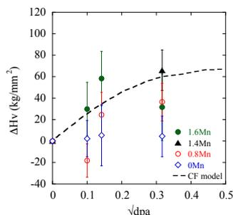
Figure 2 dpa dependence of hardness change in RPV steels containing 0%Cu, 0.8%Ni and various (0 to 1.6%) Mn irradiated by  $\text{Fe}^{2+}$  ion.
