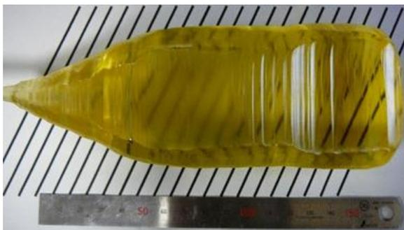
Fig.1 Novel langasite-type single crystal.
