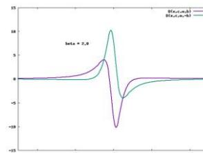
Fig.1 FMR resonance line shape for asymmetry parameter  $\beta = 0$  (green line) and 2 (violet line).
