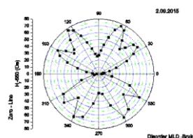
Fig. 2 Angular in-plane dependence of the FMR resonance field for asymmetry parameter  $\beta=0$  – MBE grown sample, not annealed.
