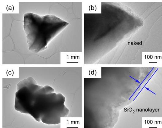
Fig. 1 TEM images of (a, b) cBN and (c, d) SiO<sub>2</sub>-coated cBN
