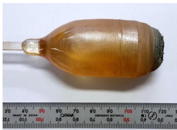
Fig. 2 As-grown  $\text{CdWO}_4$  single crystal
