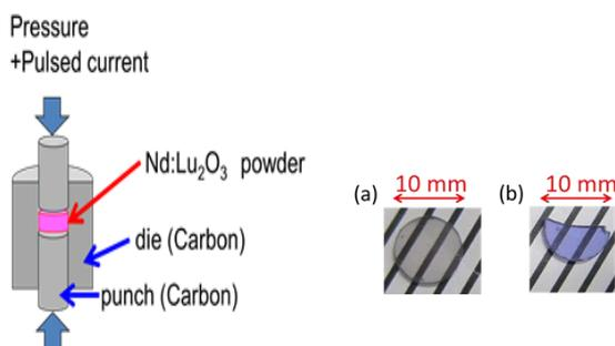
Fig. 1 Schematic view of SPS technique to fabricate Lu<sub>2</sub>O<sub>3</sub> ceramics doped with 0.1 mol% (a) and 5.0 mol% (b) of Nd (after polishing).
