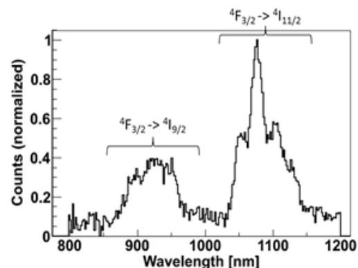
Fig. 2 X-ray-excited radio-luminescence of 0.5 mol% Nd:Lu<sub>2</sub>O<sub>3</sub> in the near infrared region corresponding to the human window.
