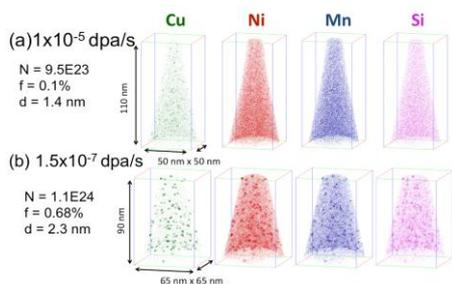
Figure 1 Atom probe elemental maps of 0.4Cu-1.3Ni-1.4Mn steel irradiated to 0.2 dpa at a)  $1 \times 10^{-5}$  dpa/s by Fe<sup>2+</sup> ions and b)  $1.5 \times 10^{-7}$  dpa/s in BR2 test reactor, showing significant delay in cluster formation at higher dose rate.
