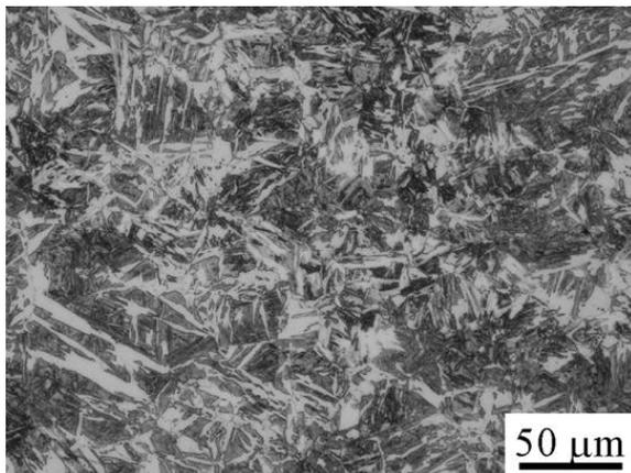
Fig. 1 Optical micrograph showing microstructure isothermally transformed for 1.8 ks at 823 K.
