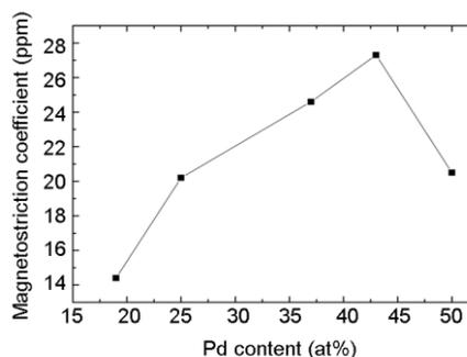
Fig. 2 Magnetostriction coefficient as a function of Pd content for  $\text{Fe}_{50}\text{Pt}_{(50-x)}\text{Pd}_x$  thin films.
