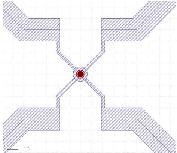
Fig. 1 Design of the quantum device fabricated in this project. The red dot represents the FePt nanopillar and the purple ring and wires represent the Ag and Cu nanowires.
