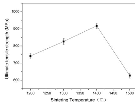
Fig.3 Variation of ultimate tensile strength with sintering temperature for T-30Ta alloy.
