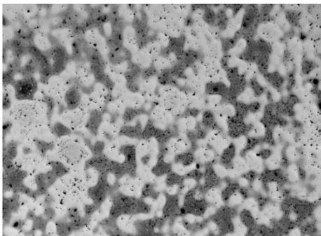
Fig.1 An OM image of typical diffusion-controlled two region structure for Ti-30Ta alloy sintered at 1400 °C.
