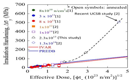
Figure 1 Irradiation hardening trend in a Cu free RPV steel.
