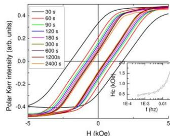
Fig. 1 Dynamic magnetization hysteresis loops of a FePt (5nm) thin film measured by PMOKE.
