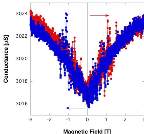
Fig. 1 Magnetoresistance of the quantum device at 350 mK.
