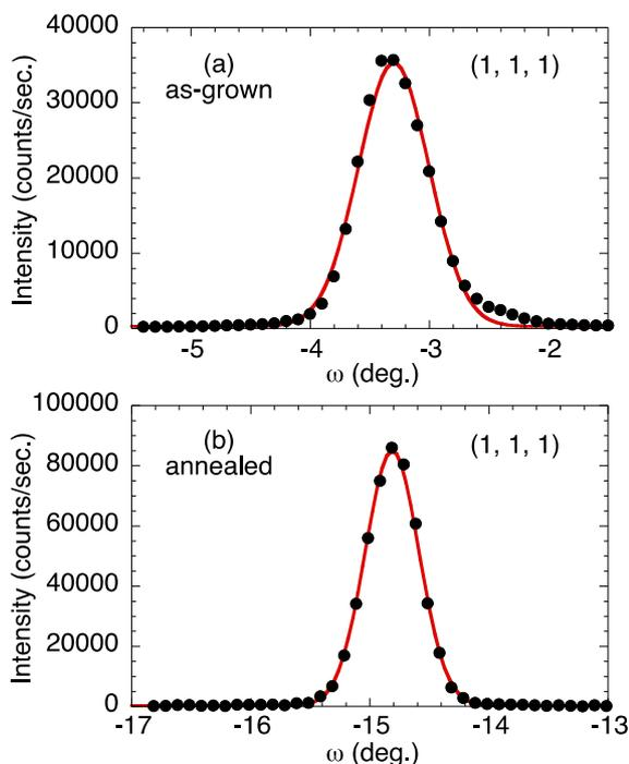
Fig. 2 Rocking curve scans of the (111) Bragg reflection in as-grown (a) and annealed crystals (b) of Heusler  $\text{Cu}_2\text{MnAl}$ . The measurements were performed using unpolarized neutrons. The solid lines are the results of fits to a Gaussian function.
