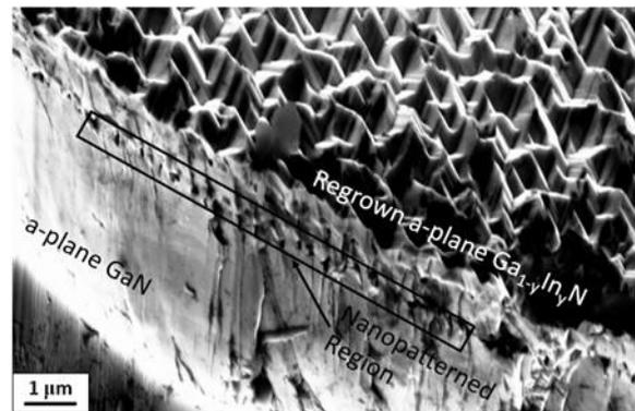
Figure 1 An SEM image showing the cleaved cross section and rough growth surface of this example of a-plane  $\text{Ga}_{1-y}\text{In}_y\text{N}$  material grown on nano patterned a-plane GaN on sapphire.
