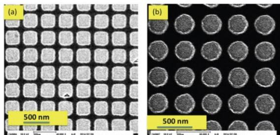
Fig. 1 Scanning electron microscopy images of FePt antidot lattices with (a) rectangular and (b) circular shapes of the holes.
