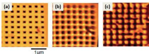
Fig. 2 (a) Morphology of a FePt antidote lattice with  $d = 200$  nm. The image shown in (b) is the magnetic domain structure taken after remanence after positive saturation. (c) Magnetic domain image taken near coercive field of  $\mu_0H = -0.15$  T.
