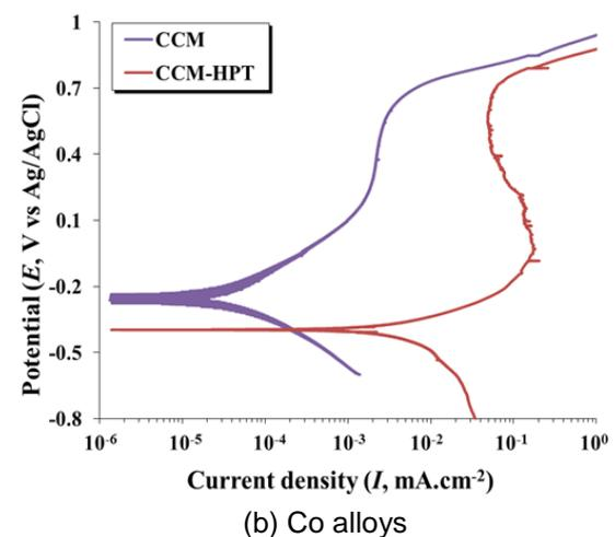
Fig. 1 Potentiodynamic polarization curves of (a) Ti alloys and (b) Co alloys
