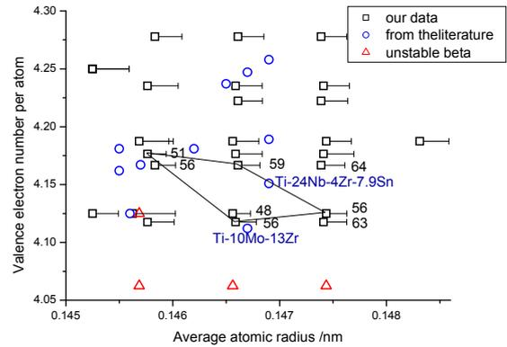
Fig. 1 Compositions of low-E alloys in a 2D map coordinated by valence electron concentration and atomic size. The data are both from our experiment ( $\square$ ) and from the literature ( $\circ$ ). The non-BCC alloys are marked with  $\triangle$ . The Young's moduli  $E$  below 65GPa are shown near the alloy compositions.
