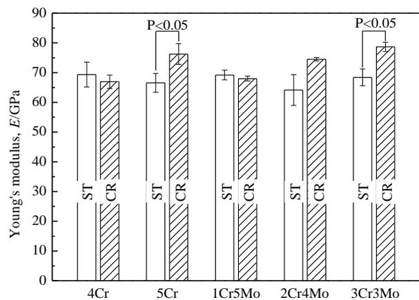
titanium alloys. Therefore, the increasing of Young's moduli in 5Cr, 2Cr4Mo, and 3Cr3Mo after cold rolling are attributed to the deformation-induced  $\omega$  phase.
