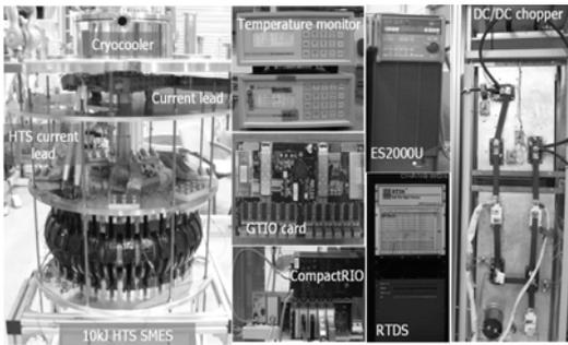
Fig. 5. 10kJ toroid-type HTS SMES and DC/DC chopper
