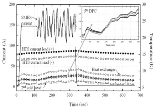
Fig. 7. Variations in the temperature of the SMES due to the operating current variations during compensating the fluctuation of utility frequency
