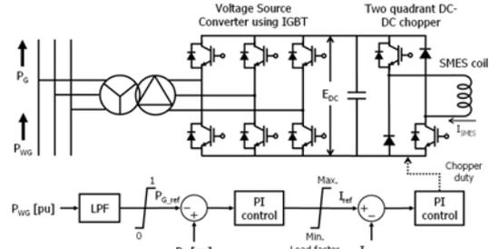
Fig. 2. Simulation circuit in PSCAD/EMTDC: Control diagram of DC/DC chopper for SMES system
