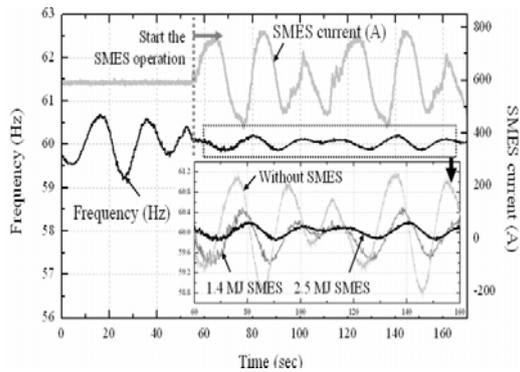
Fig. 6. Utility frequency stabilized by the SMES system and the variation in the current of the SMES using PHILS technology
