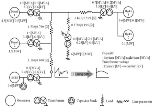
Fig. 1. Schematic diagram of the model power network including WPGS
