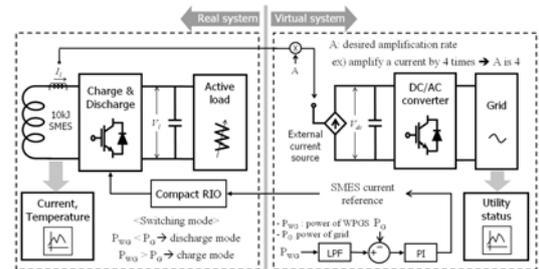
Fig. 4. Conceptual diagram of PHILS with RTDS and a real HTS SMES
