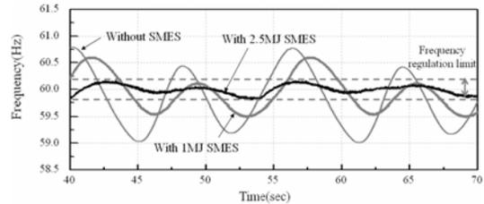
Fig. 3. Comparison of load side frequency stabilized by 1 MJ and 2.5 MJ SMES systems
