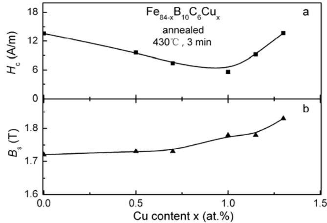
Fig.3. Cu content  $x$  dependence of (a) coercivity  $H_c$  and (b) saturation magnetic flux density  $B_s$
