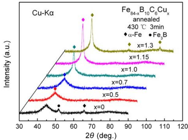
Fig. 1. X-ray diffraction patterns for annealed  $\text{Fe}_{84-x}\text{B}_{10}\text{C}_6\text{Cu}_x$  alloy ribbons
