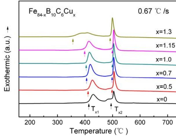
Fig.2. DSC curves for  $\text{Fe}_{84-x}\text{B}_{10}\text{C}_6\text{Cu}_x$  melt-spun ribbons
